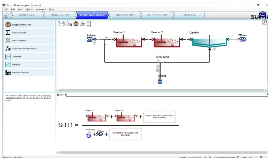
Figure 6 - SRT calculation setup
