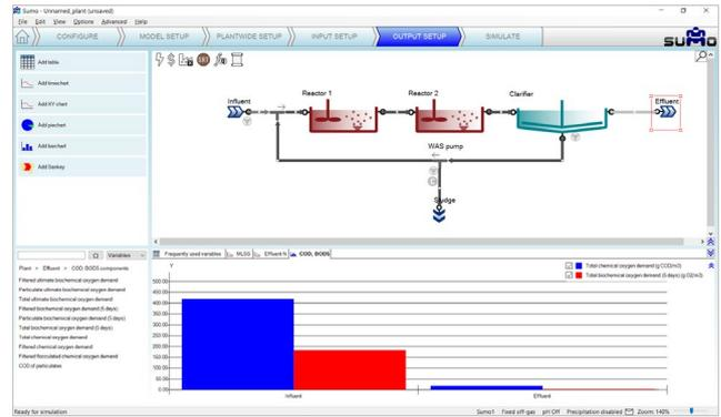
Figure 11 - COD/BOD5 removal setup
