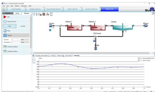
Figure 21 - Wastage timechart with measured data
